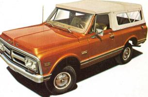
The JIMMY Soft-Top is a dealer-installed accessory that folds down like a convertible top or remains extended with sides rolled up. Preshrunk fabric is vinyl coated and treated for lasting appearance. Heat-sealed windows keep moisture out. Adds fun to any JIMMY experience!
