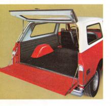
Wide-Opening Lockable Lift and Tailgate with room for wide, bulky loads swings open for easy and convenient oading. Spare wheel, tire and stand unpolt for extra room. Telescoping supports hold liftgate securely in open position.
